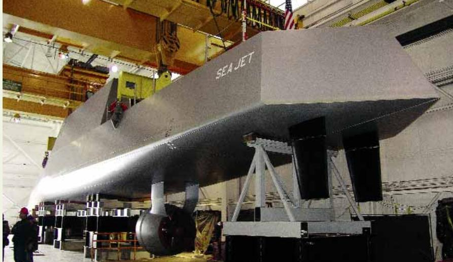
*A view of RimJet installed on the Navy's Advanced Electric Ship Demonstrator vessel SEAJET.*
