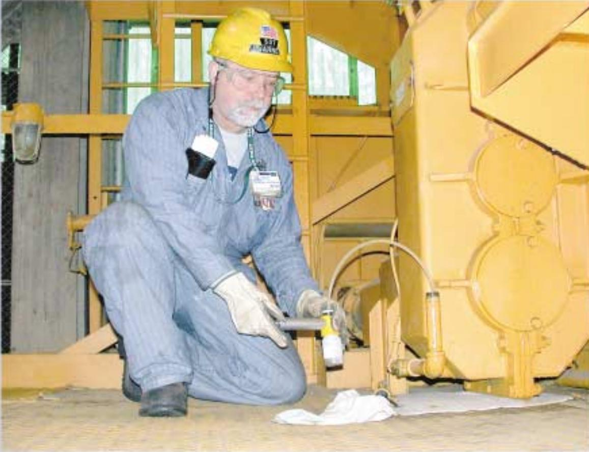
*Mechanical services engineer John Warner (507) takes an oil sample from one of the two heavy lift bay cranes in Building 260.*
