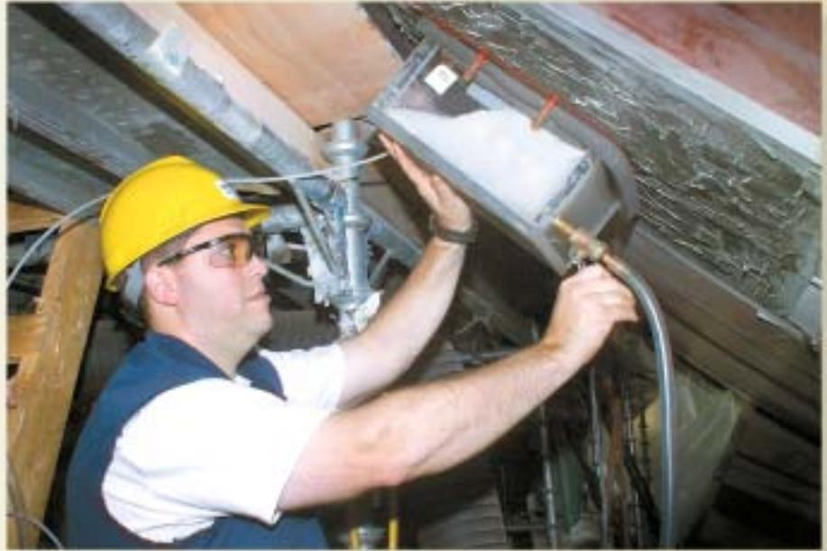
*Using a new test device that he developed, STO electrical test technician Mike Appio (272) prepares to evaluate the Virginia's (SSN-774) hull corrosion-prevention system by filling the device with a saltwater solution.*
