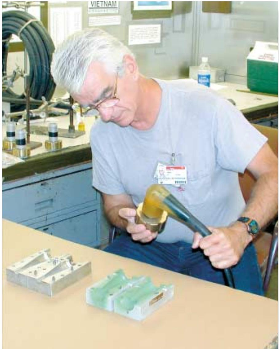
*Vulcanizing technician Ed Frink holds a finished polyurethane electrical connector, which now features the part number etched into the metal rim. In front of him are two of the molds used to create the connectors. The green one is Teflon-coated.*
