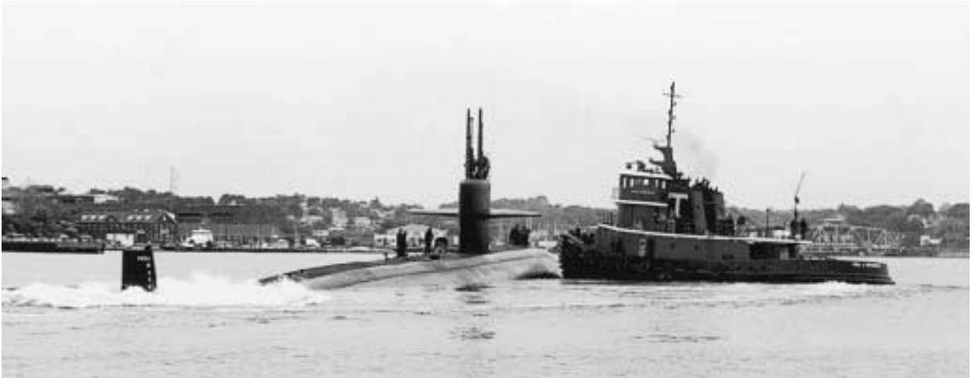
At the completion of its SRA sea trial and after EB ship riders transferred to the tug, USS Dallas (SSN-700) is turned around in the Thames River before heading out to sea.
