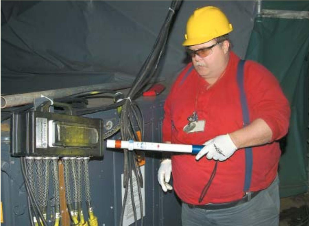
*Bob Mashuta (241) demonstrates the use of an AC Hot Stick, a tool that can check electrical cables for current without having to touch them.*
