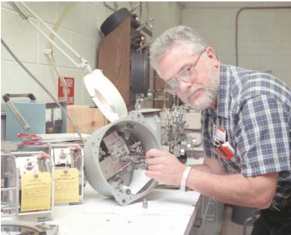
Metrology Lab employee Keith Gould (341), who works at the sub base's Naval Submarine Support Facility, holds a disassembled depth gauge.
