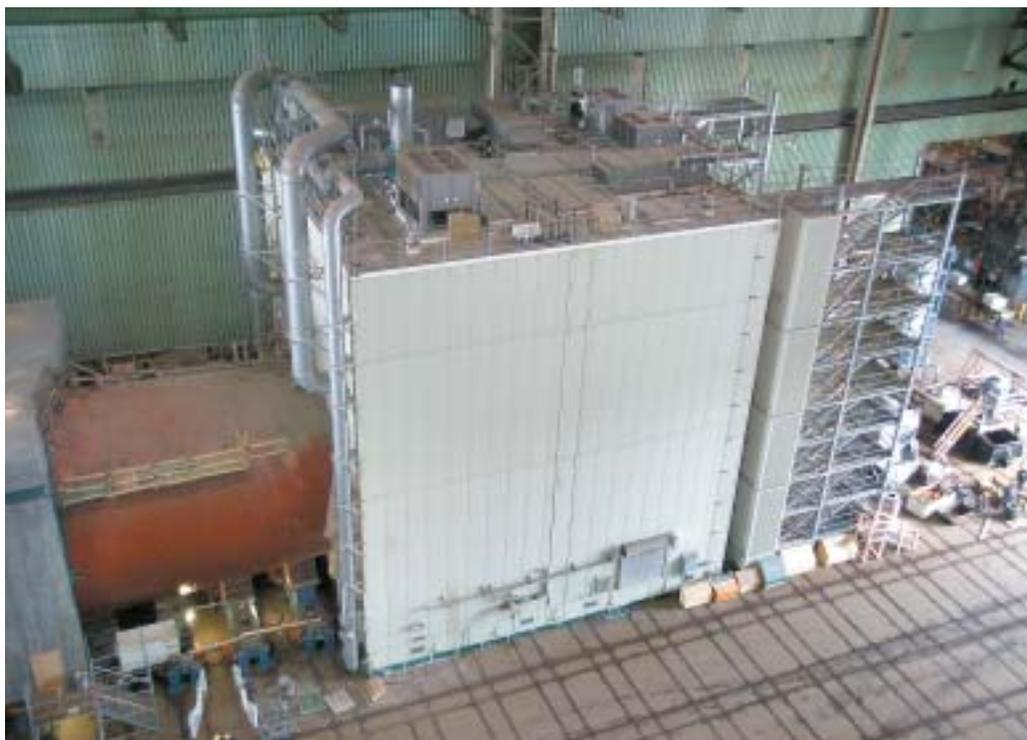
*Electric Boat's new MIP enclosure is ready for its first Mold-In-Place tile installation and pour.*
