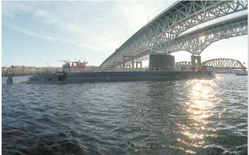
THE HISTORIC SHIP NAUTILUS passes beneath the Gold Star Bridge earlier this month on its way to Electric Boat for a \$4.7 million Preservation Availability. EB will blast and paint exterior surfaces, repair deteriorated sections of the exterior structure and replace the wooden decking. The job is scheduled for completion in May.
